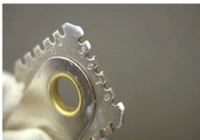
The purpose of measuring coating thickness on concrete is to control coating costs while ensuring adequate protective coverage. Shown here is a wet-film thickness gage. Photo courtesy of KTA-Tator Inc.
