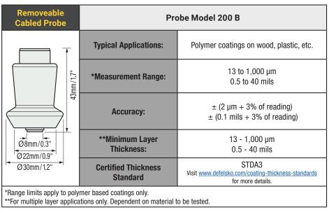
200 B probe measures coating thickness over wood, plastic, and other non-metal substrates using ultrasonic technology.
