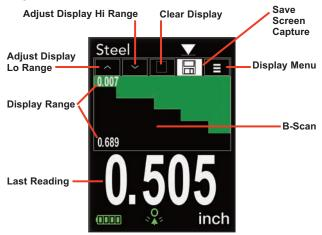
Adjust Display Lo/Hi Range - Adjusts the minimum and maximum displayed range for the B-Scan. Use the (-) and (+) buttons to decrease/increase gain. Note: This does not alter the instruments measuring range.
