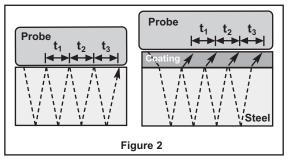
In the figure above, multiple-echo mode measures only the time between echoes. Regardless of whether the steel is coated or not, all times between echoes are the same. In multiple-echo mode the gage determines thickness by measuring  $t_1 + t_2 + t_3$ , dividing it by six and then multiplying by the velocity of sound for that material.
