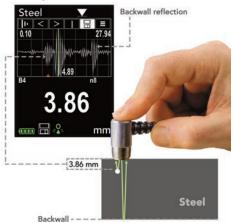
**PosiTector UTG M** and **PosiTector UTG P** probes provide two cursors (vertical green lines) which allow the user to measure the difference between echoes shown in the graphic display.
