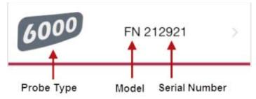
**NOTE:** The PosiTector App features probe hot-swap. During the measurement process, probes can be interchanged without the need to go back to the search screen. Simply swap probes (PosiTector *SmartLink* will power-down) and then power-up the PosiTector *SmartLink*. The PosiTector App will automatically recognize the probe and be ready to measure.
