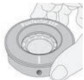
The **PosiTector SST** can be used as a conventional conductivity meter making it ideal for testing abrasive materials in accordance with ISO 11127-6 and ASTM D4940-15. See **Bresle Mode** (pg. 10).
