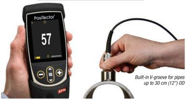
When attached to either a PosiTector Standard or Advanced body, the **PosiTector** *SPG OS* probe measures the peak-to-valley profile height of flat or convex abrasive blast cleaned surfaces.
