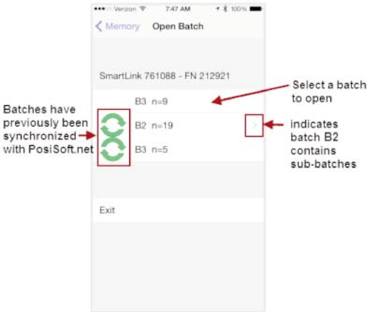
Additional measurements can be added to existing batches only if the original probe is attached to the PosiTector *SmartLink*.
