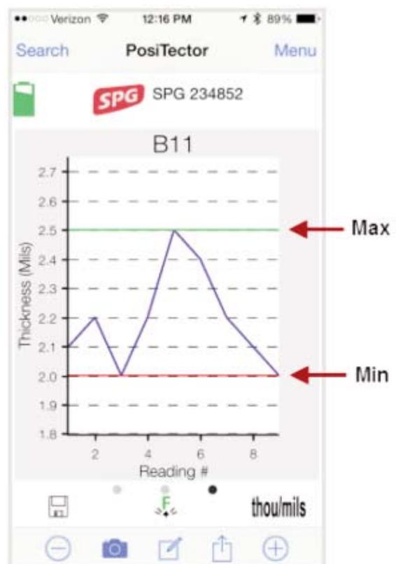
**New Sub-Batch** (*appears only if a batch is currently open*)
