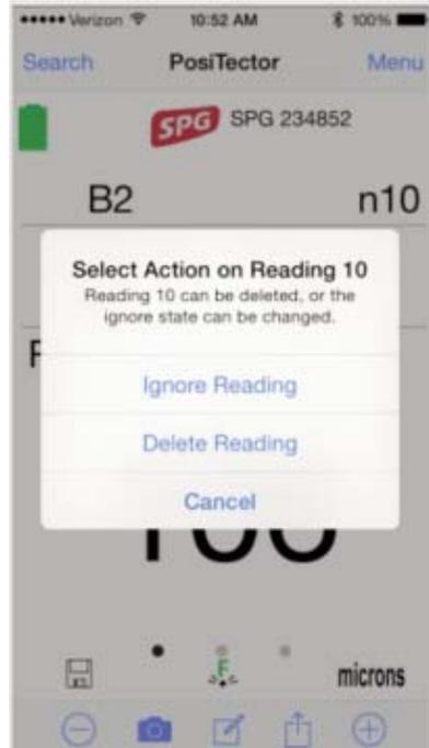
By default Ignored Readings are not included on reports. For inclusion, toggle the Hide Ignored Readings within the *Batch Report Configuration* (pg 20). Ignored Readings will display as highlighted within the readings section of the report, but are excluded from the statistical summary and chart.
