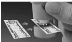
To position the tape, align the two dots (printed on replica tape) with arrows on both sides of the measurement opening.
