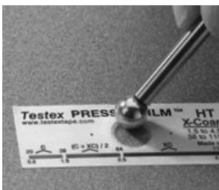
Pull a single adhesive-backed replica tape free of its release paper. A "bull's eye" circle of paper should remain on the release paper (it is not used for measurement).
