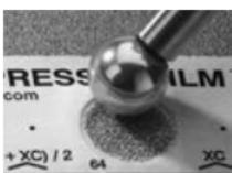
Firmly compress the foam using the rounded end of the included stainless steel burnishing tool. Apply sufficient pressure in a circular and x-y rubbing motion to produce a replica with a uniform pebble grain appearance. **Excessively hard rubbing should be avoided because the polyester film could become distorted.** It normally takes 30 to 60 seconds to fully compress all parts of the foam on most surfaces. After burnishing is complete, remove the replica tape from the surface.
