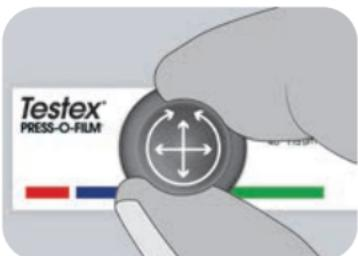
5. Alternate between linear (x-y) and circular motions with the burnishing tool to completely burnish the replica foam until a uniform stippled gray appearance is achieved across the entire measurement area.
