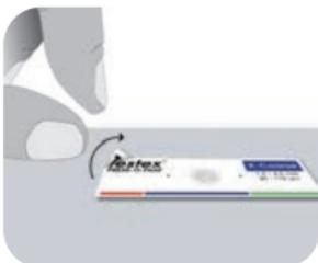
7. Inspect the replica to ensure that no contamination from the surface is present (e.g. dust, debris, residual blast media).
