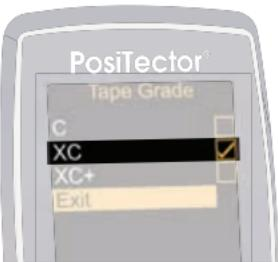
9. Ensure the correct grade of replica tape is selected (pg. 3) and the **HL** icon (pg. 9) is displayed at the bottom of the screen.
