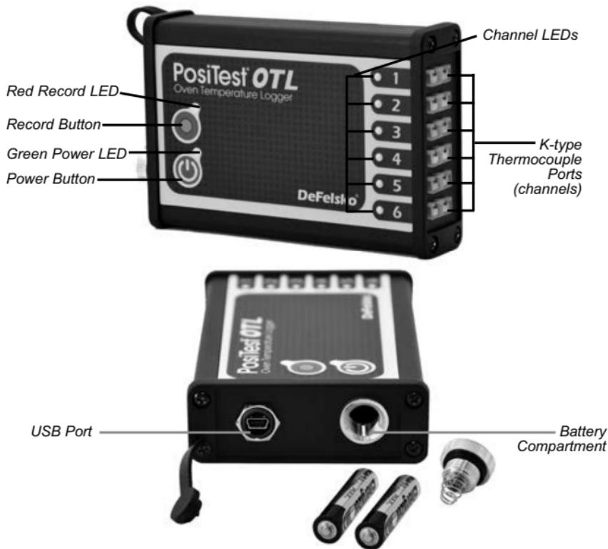
Basic operating instructions are located on the back panel of the **PosiTest OTL**.
