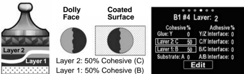
Cohesive and adhesive fractures are identified as follows:
