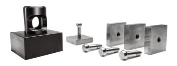
The **PosiTest** *AT 50 mm x 50 mm Tile Kit* is designed to measure tensile strength of ceramic tile cementitious, dispersion and reaction resin adhesives in accordance with BS FN 12004-2
