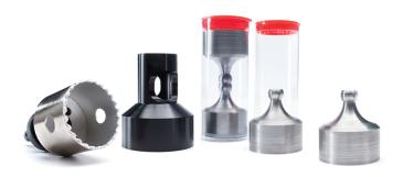
The **PosiTest** *AT 50 mm C1583 Kit* is designed to measure tensile strength of concrete surfaces and the bond strength or tensile strength of concrete repair and overlay materials by direct tension (Pull-Off Method), in accordance with ASTM C1583.
