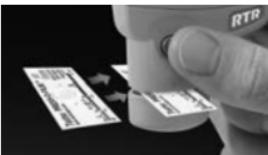
To position the tape, move the tape to the back of the probe and align the two dots (printed on replica tape) with arrows on both sides of the measurement opening.
