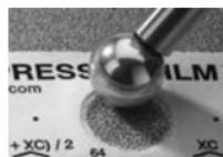
**Excessively hard rubbing should be avoided because the polyester film could become distorted.** It normally takes 30 to 60 seconds to fully compress all parts of the foam on most surfaces. After burnishing is complete, remove the replica tape from the surface.
