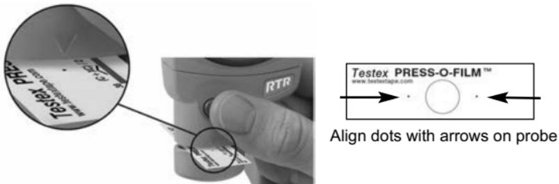
Align dots with arrows on probe
