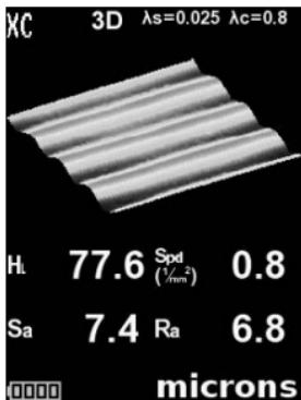
**NOTE:** Press the Up navigation button to toggle between 2D and 3D images if the image does not automatically appear on the display.
