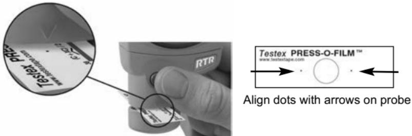
If you are using older tape that does not have the printed dots, simply align by centering the tape within the measurement opening.
