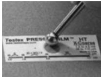
Firmly compress the foam using the rounded end of the included stainless steel burnishing tool. Apply sufficient pressure in a circular and x-y rubbing motion to produce a replica with a uniform appearance.
