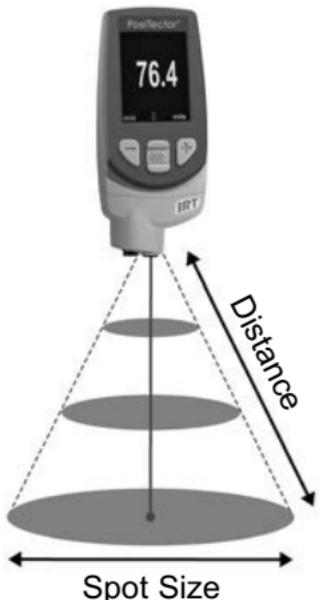
The distance to spot ratio refers to the relationship between the diameter of the area being measured compared to the instrument's distance from the area. As the distance (D) from the target increases, the spot size (S) of the area being measured by the unit becomes larger. The D:S ratio of the **PosiTector IRT** is 5.7:1. For example, when the instrument is 100 cm (40 inches) from the target, the spot size will be about 18 cm (7 inches) in diameter.
