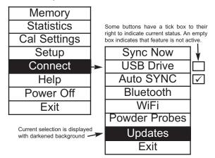
To navigate, use the Up and Down buttons to scroll vertically and is SELECT.
