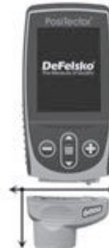
The **PosiTector** gage body accepts a wide variety of probe types including magnetic, eddy-current, and ultrasonic coating thickness, surface profile, environmental, hardness, salt contamination, gloss, and ultrasonic wall thickness probes. See [www.defelsko.com/probes](http://www.defelsko.com/probes)
