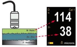
N = Paint ThicknessZn = Zinc Thickness
