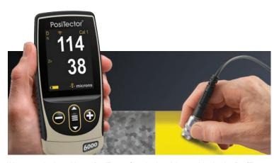
When attached to either a PosiTector Standard or Advanced body, the **PosiTector** *6000 FNDS* probe measures the individual thicknesses of both the paint and the zinc layers in a duplex coating system with a single reading.
