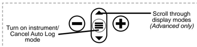
**Standard models** remain powered-up while in auto log mode. The instrument will take readings for 50-60 hours on a set of alkaline batteries, depending on the frequency of measurements.
