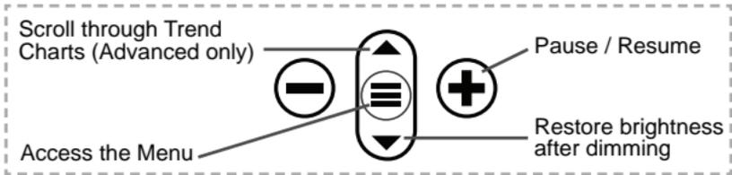
The Pause/Resume (+) button stops values from automatically updating to allow for closer examination of the relationship between the values or to allow time to manually record the entire dataset. Press (+) again to resume.
