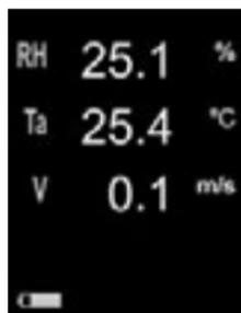
**NOTE:** Dew point (Td) and surface temperature (Ts) are not displayed when the **Anemometer** is enabled.
