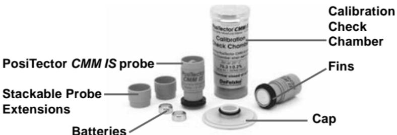
**NOTE:** For instructions on how to use the **PosiTector CMM IS** and the **PosiTector App** in accordance with ASTM F2170, refer to **Setting Up a New ASTM F2170 Project** (pg. 6).
