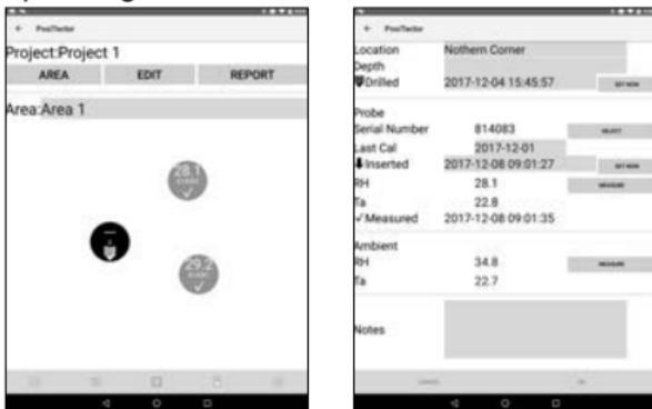
Ambient Relative Humidity and Air Temperature (above the hole) can be recorded using a spare **PosiTector CMM IS** probe or **PosiTector DPM Advanced** instrument. The ambient instrument being used is specified within the **Project setup** (pg. 6). Select Measure, and then Ok to store the displayed values. Alternately, a relative humidity and temperature value can be entered manually.
