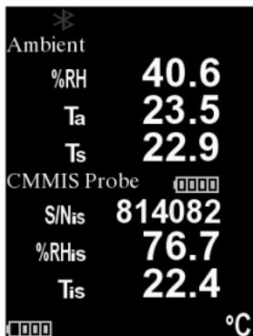
To record, ensure a batch is open in memory and press the (+) button on the gage. The displayed readings of the PosiTector DPM probe and the PosiTector CMM IS probe will be recorded into the gage's memory. If a batch is not currently open, select **New Batch** from the gage's Memory menu. To add measurements to an existing batch, select **Open** from the gage's **Memory** menu.
