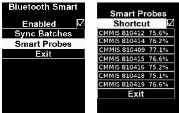
3. The relative humidity and temperature measured by the PosiTector CMM IS probe will be displayed below the ambient relative humidity, air temperature and surface temperature measured by the PosiTector DPM probe, as shown below:
