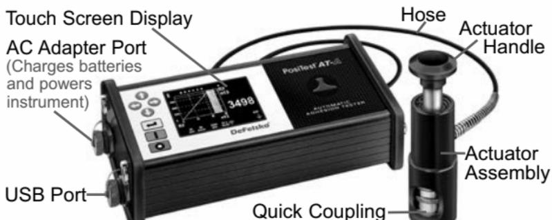
The **PosiTest AT-A** powers up when the button is pressed. To preserve battery life, the instrument powers down after 5 minutes of no activity. Alternatively, press and hold the button for 5 seconds or select *Power Off* from the menu.
