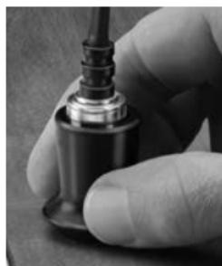
Verify accuracy (pg. 4) at the beginning and the end of each shift, or if the gage is dropped or suspected of giving erroneous readings.
