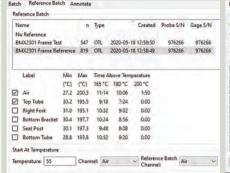
**Reference Batch**—store optimal cure reference profiles to compare measurement results
