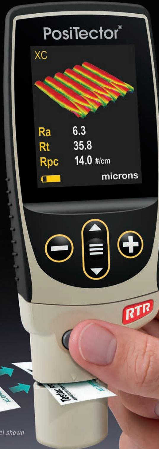
Measures and records surface profile parameters using replica tape
