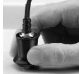
A second reading may be taken at the same spot by continuing to hold the probe down on the surface.
