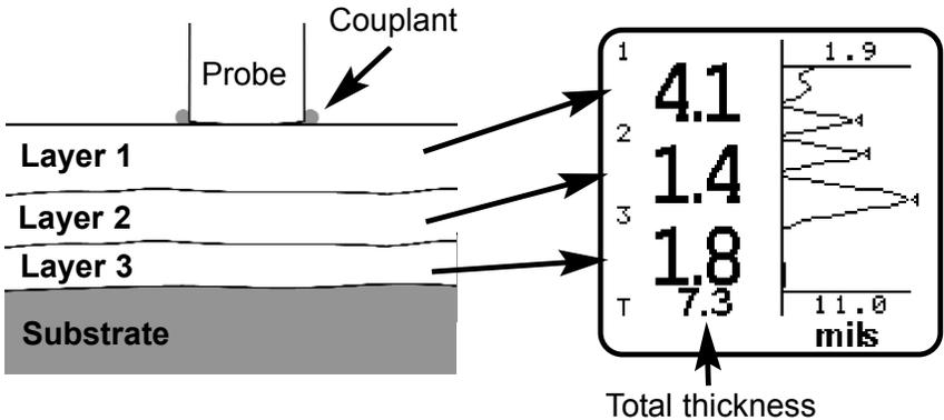
To setup the Gage for multi-layer coatings:
