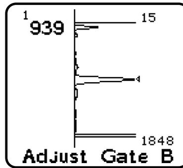
For most applications the default Gate values do not have to be adjusted. But some conditions may exist in the user's application that cause the Gage to display very low or non-repeatable readings. These conditions include...
