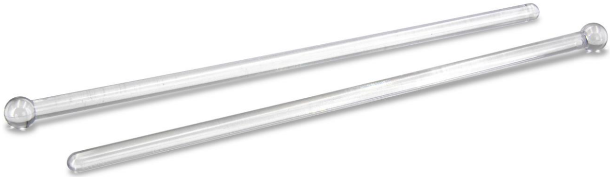
Figure 4: The burnishing tool currently used for the replica tape method
