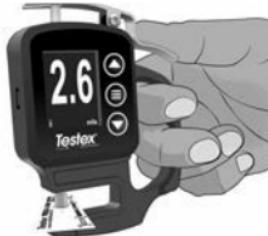
Once the measured value stabilizes, the displayed value will flash, and be recorded if Memory Mode is enabled (pg. 6).
