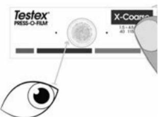
7. Inspect the replica to ensure that no contamination from the surface is present (e.g. dust, debris, residual blast media).
