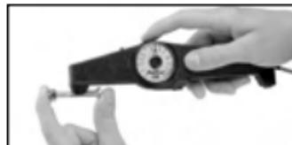
B. Never verify accuracy on shim stock. Verification is best achieved by using coated metal plate standards.
